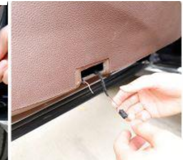
4. The red line is connected to the positive wire. Connect the black wire to the negative wire.
