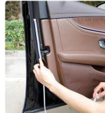
1. Tear around the edge of the door.
