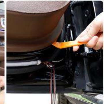
2. Pry open the gap at the bottom of the door.
